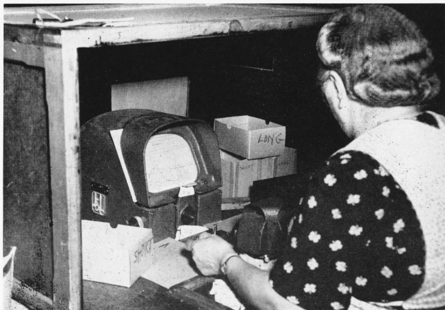
Martha Buchs gauges screw machine products on one of the Screw Machine Inspection comparators. A glance at the screen of the comparator tells Martha whether or not the piece of work falls within the tolerances specified by the blueprint or whether it is oversized or undersized.
